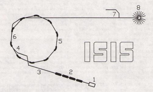
1. ION SOURCE AND PRE-INJECTOR - The protons begin their journey towards the target as the nuclei of negatively charged Hydrogen ions (H<sup>-</sup>). These are produced in a Penning type ion source by bombarding a Caesium coated surface with positive and neutral ions from a Hydrogen discharge. The H<sup>-</sup> current required for full output is 40mA at a duty cycle of 2½% (50Hz X 500µs).
