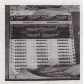
The results of the Division's work have also been used in Space Science research. Here is shown a module which is set to fly in the forthcoming ATSR satellite.
