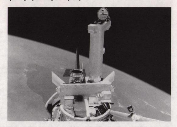
The picture shows the payload bay viewed from the flight deck of Challenger. The IPS and its complement of experiments are pointing at the sun.
