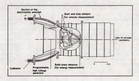
Sketch of the Magnetospheric Ion Composition Spectrometer for CRRES
