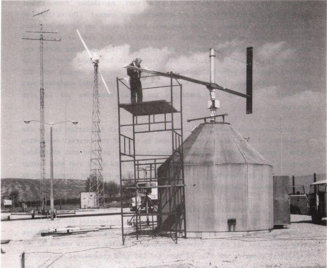
Figure 1. A typical scene at RAL Wind Turbine Test Site. In the foreground lies an early version of the Musgrove vertical axis machine and in the background a modern horizontal axis machine.
