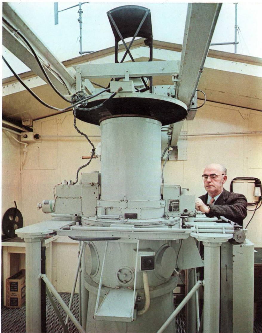
Left: Preparing the photographic zenith tube for a night's work.
