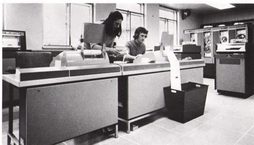
The Observatory is equipped with an ICL 1903 T computer. Such a powerful machine is required to prepare the Nautical Almanac and to handle the large amounts of data produced by the measuring machines.
