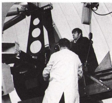
Engineers replacing the Cassegrain secondary mirror after the completion of a run with the coudé spectrograph.
