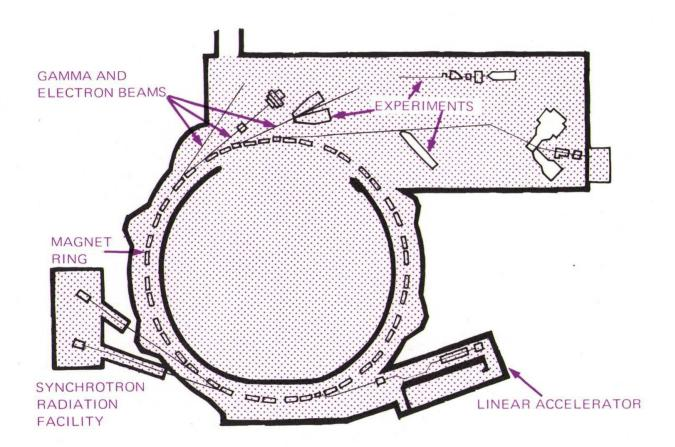
The electrons can be extracted from NINA for use in high energy physics experiments. Alternatively they may be allowed to strike a thin metal plate in order to produce photons (gamma rays) for use in the experiments. The electrons or photons are made to collide with a
