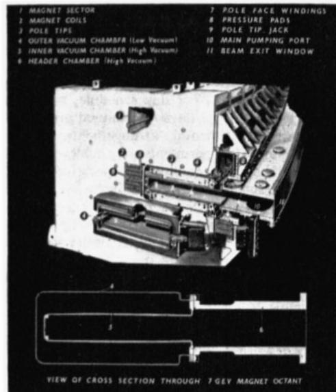
Figure 3. Section through NIMROD magnet.
