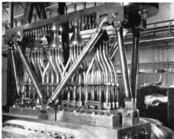
Figure 6. Body of National liquid hydrogen bubble chamber, showing part of expansion system.
